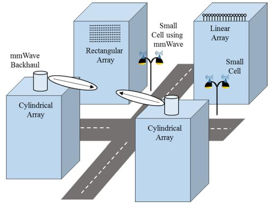
Figure 1. A possible 5G green networking deployment scenario in which different massive MIMO configurations and an underlay of dense small cell deployment, some of which transmit on the mmWave, are depicted.
