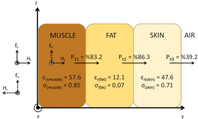
Figure 7.4: Multi-layer human tissue model at 403 MHz ( $\epsilon_r$ : Permittivity,  $\sigma$ : Conductivity,  $P_\tau$ : Power transmission factor). ©2016 IEEE. Reprinted with permission from [57].
