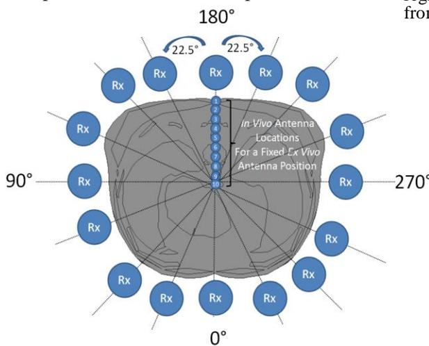
Figure 7.9: *In vivo* and *ex vivo* antenna locations in the simulation. 16 (angles) x 10 (depth) x 4 (regions) = 640 simulations are performed for path loss in total. ©2014 IEEE. Reprinted with permission from [45].
