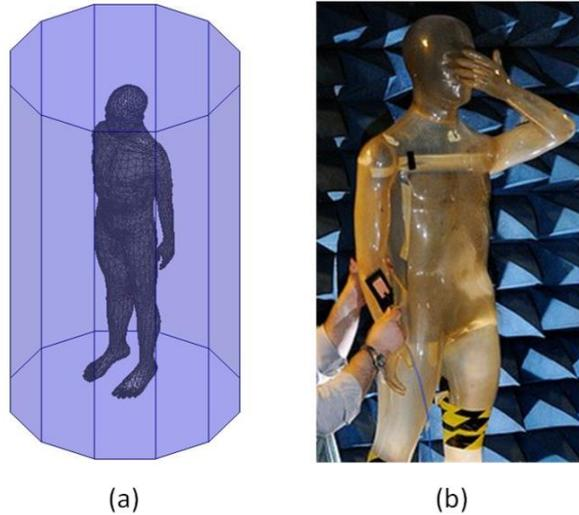
Figure 7.3: Heterogeneous human body models: (a) HFSS<sup>®</sup> model [19] (b) physical phantom [14]. ©2016 IEEE. Reprinted with permission from [57].
