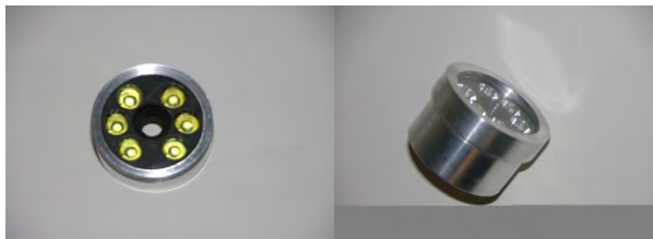
Figure 3. Assembled heat sink, reflector array and LED ring
