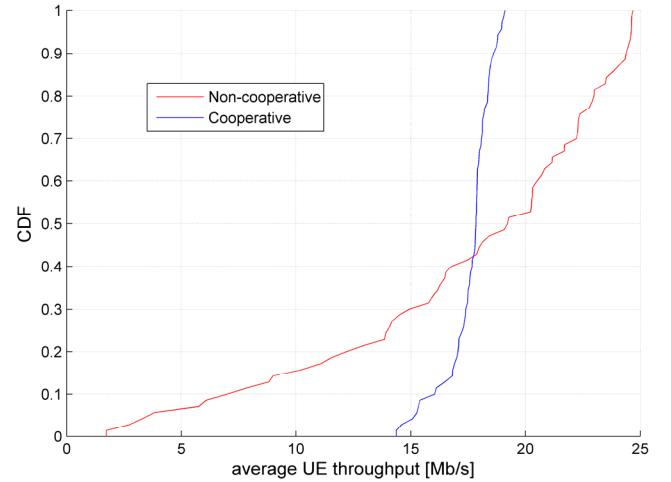
Fig.4. UE throughput CDF for non-cooperative and cooperative massive MIMO with 50 transmit antennas.
