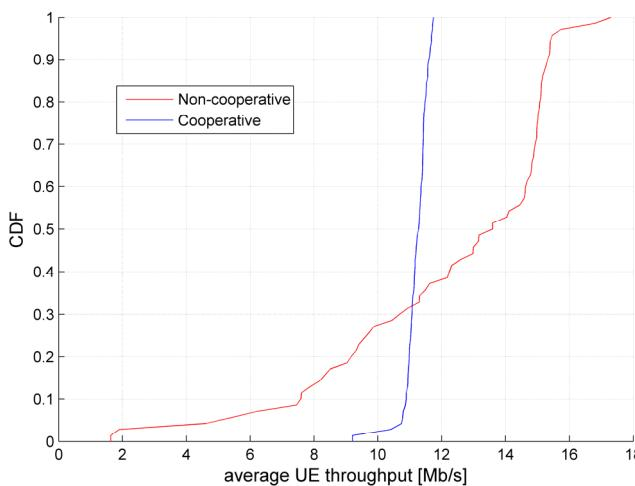
Fig.3. UE throughput CDF for non-cooperative and cooperative massive MIMO with 25 transmit antennas.
