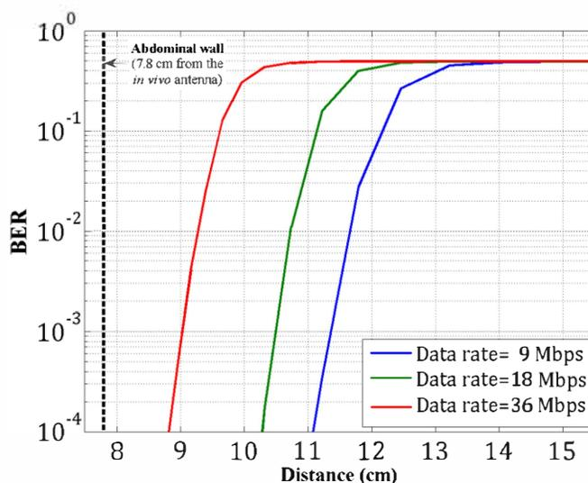
Figure 4. BER performance as function of distance for different data rates at the threshold power (0.412 mW).
