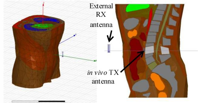
Figure 2. Truncated HFSS human body model used to derive SAR levels and channel model (left). Cross section of same model showing receive and transmit antenna locations (right).
