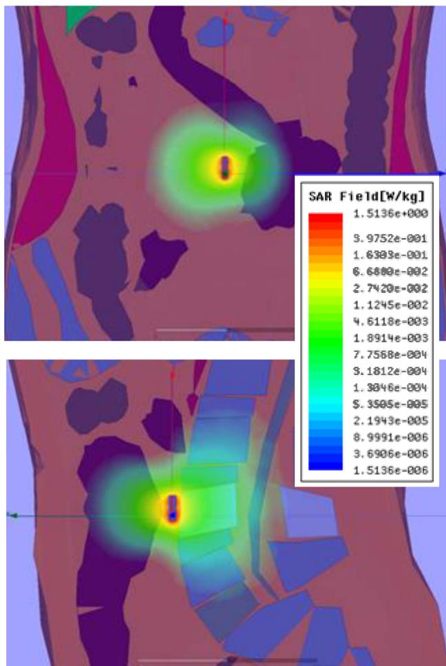
Figure 3. Front (top) and Side (bottom) cross-sectional views of the total SAR generated at 2.412 GHz inside the abdomen at a transmit power of 0.412 mW.
