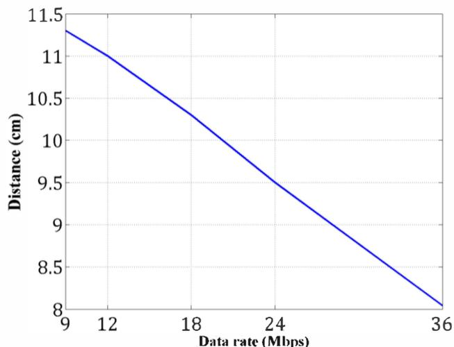
Figure 5. Achievable distance, as a function of bit rate, between *in vivo* and external antennas for a BER of 10<sup>-6</sup>.
