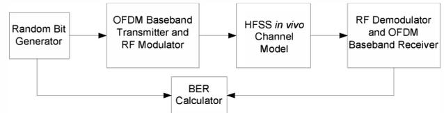
Figure 1. Block diagram of system level simulation showing direct link to the HFSS *in vivo* channel model.
