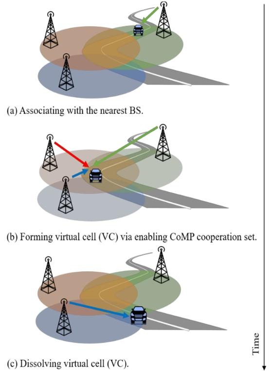
Fig. 1: Adaptively enabling / disabling coordinated multipoint (CoMP) transmission according to the trajectory of user in the network. (a) Associating with the nearest base station (BS). (b) Forming a virtual cell (VC) via enabling CoMP cooperating set. (c) Dissolving a VC.
