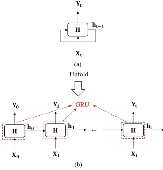
Fig. 3: (a) The structure of a conventional RNN. (b) The unfolded RNN structure in time when using the GRUs in the hidden layers.
