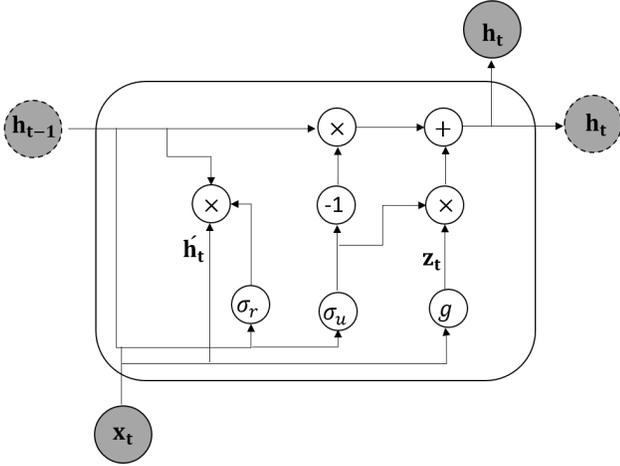
Fig. 4: Gated Recurrent Unit (GRU) architecture. Dark gray circles with a solid line are the variables whose content is exchanged with the input and output of the network. Dark gray circles with a dashed line represent the internal state variables, whose content is exchanged within the cells of the hidden layer. White circles with  $+$ ,  $-1$  and  $\times$  represent linear operations.
