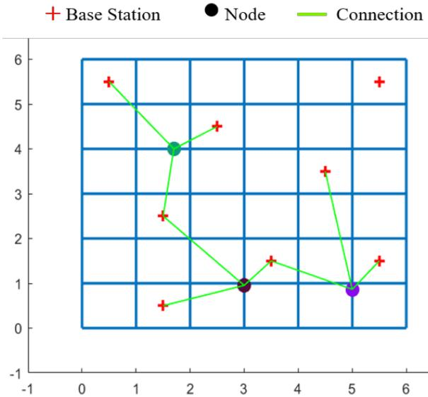
Fig. 2: A road network with eight base stations (BSs) (crosses) and a mobile node (circle). The grid lines are the roads. Each mobile node measures the received signal strength (RSS) from the three closest BSs.
