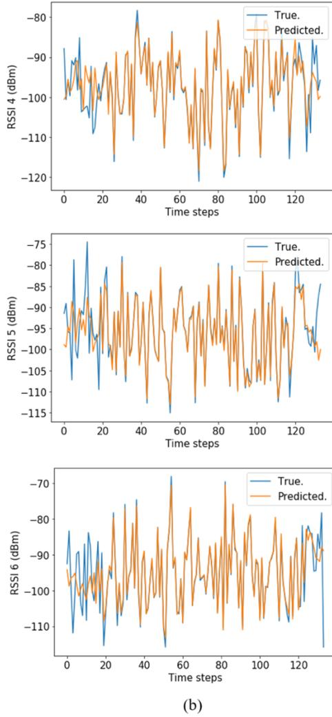
Fig. 5: True versus predicted Received Signal Strength (RSS) values for two different UE. (a) True and predicted RSS values measured from closet three BSs (3, 4 and 5). (b) True and predicted RSS values measured from closet three BSs (4, 5 and 6).
