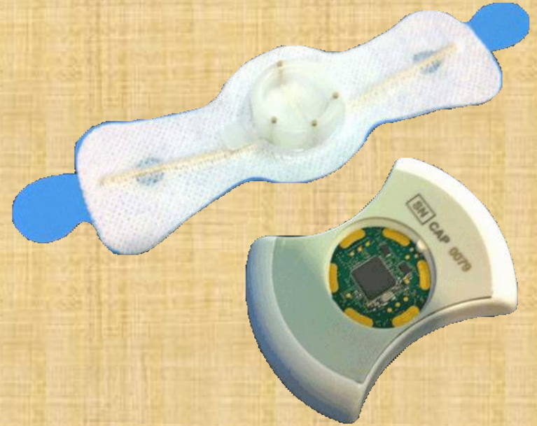
A low-power ECG patch made by imec
